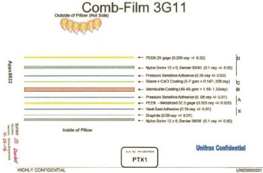
Appellee Br. 10; J.A. 8033. The refractory layer in Combi-Film 3G11 consists of an HTS-SE vermiculite dispersion containing vermiculite, a material known as DEHESIVE 480, tetrasodium pyrophosphate, and water.
